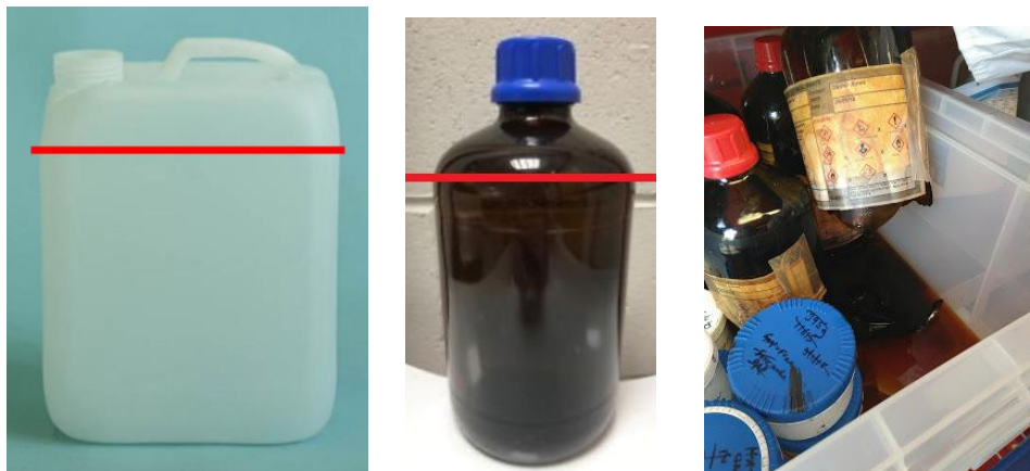
Figure 2. Maximum fill height of a waste container and the consequences of overfilling and incorrect use of glass Winchesters.
