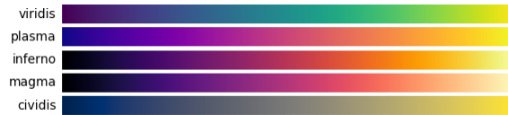
Figure 24: Image of several the commonly used continuous colour maps, where colours on the right and left hand side of each represent the minimum and maximum data range of whatever value they are being mapped to respectively.
