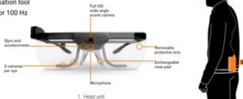
Figure 3.9: Tobii Pro Glasses 2 consisted of the head unit that is wearable eye-tracking glasses and the recording unit connected to the head unit. Image of Tobii Pro Glasses 2 has been utilised from [78].
