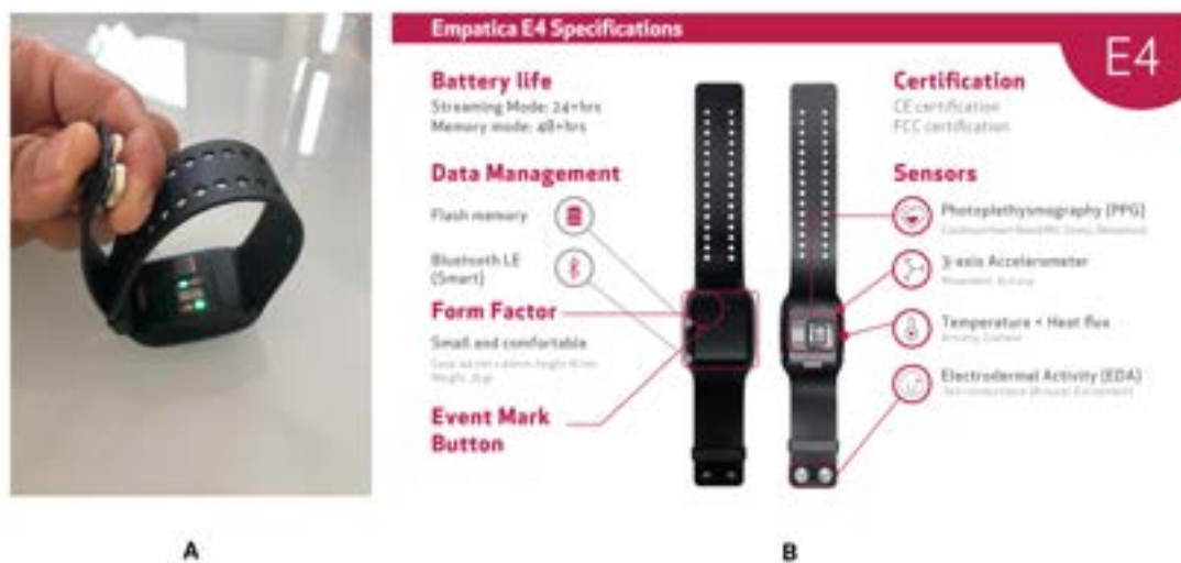
Figure 3.10: Empatica E4 wristband and its specification. Image of E4, Fig. 3.10 (A) has been utilised from [80]. Image of Empatica E4 Specification, Fig. 3.10 (B) has been utilised from [81].
