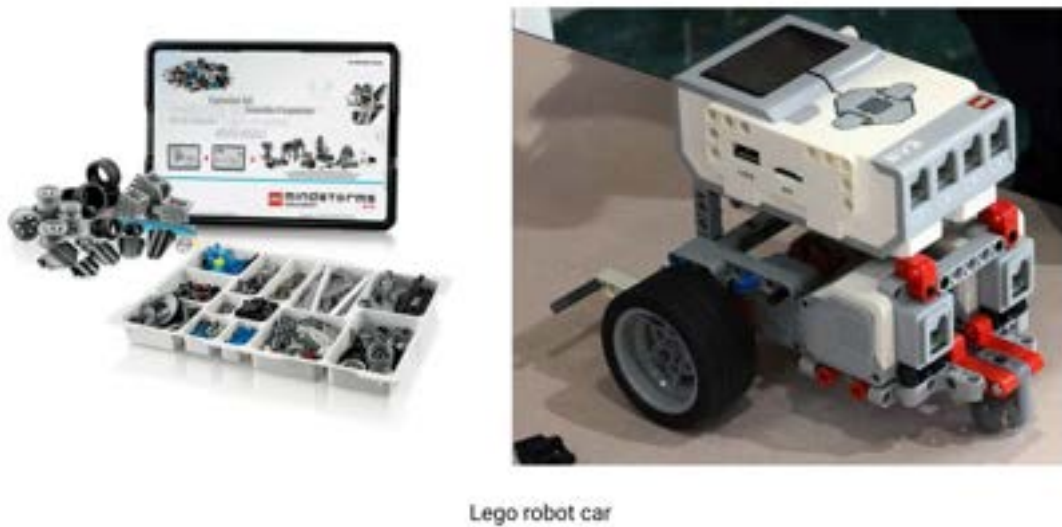
Figure 3.4: Lego Robot Car is manufactured by Lego as part of the LEGO MINDSTORMS Education EV3 set. The set includes various elements such as structure, connector, and movement that can be used to build a form. Hence it is modular and different elements could be opened up and re-joined. We used this activity after discussing it with the field experts and industry experts. The Lego Robot car allows capturing how the user assembles the different parts and how the form is broken up. Image of Lego Robot Car has been utilised from [66].
